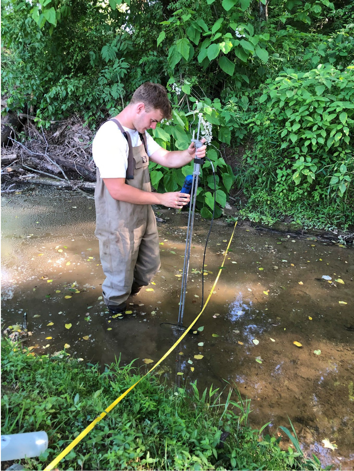
Figure 11. An Ecosystems Connections Institute intern taking a stream discharge measurement at a tributary of West Boggs Lake on 14 June 2021.
